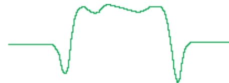
AV-1a Phase Sensitive Slice Plot – Surround out of Phase
