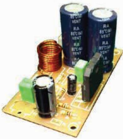
Figure 5. The LM3886 IC U1 must be soldered so that it is standing close to 90 degrees relative to the PCB surface. The rear tab of the IC will line up with the edge of the PCB. This will minimize undue stress when you mount U1 later in a heat sink.
