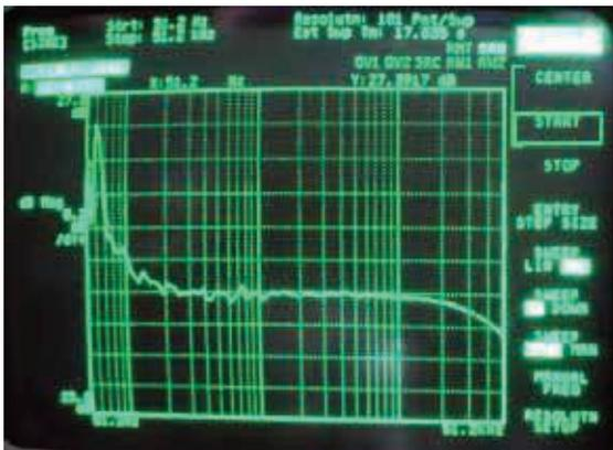
Figure 8. Photo of LM3886 Kit Magnitude response curve as plotted by HP35665a. A 1dB peaking occurs at around 60Hz. Gain is measured at 26.6dB with +/- 0.2dB flatness from 100Hz to 50KHz.
