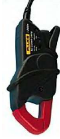
Fluke 1200s Current Clamp 0.1 to 24 A @ 100mV and 0.5 to 240 A @ 10mV/A 40Hz - 10Hz BNC or twin banana plug output Max test conductor 20mm
