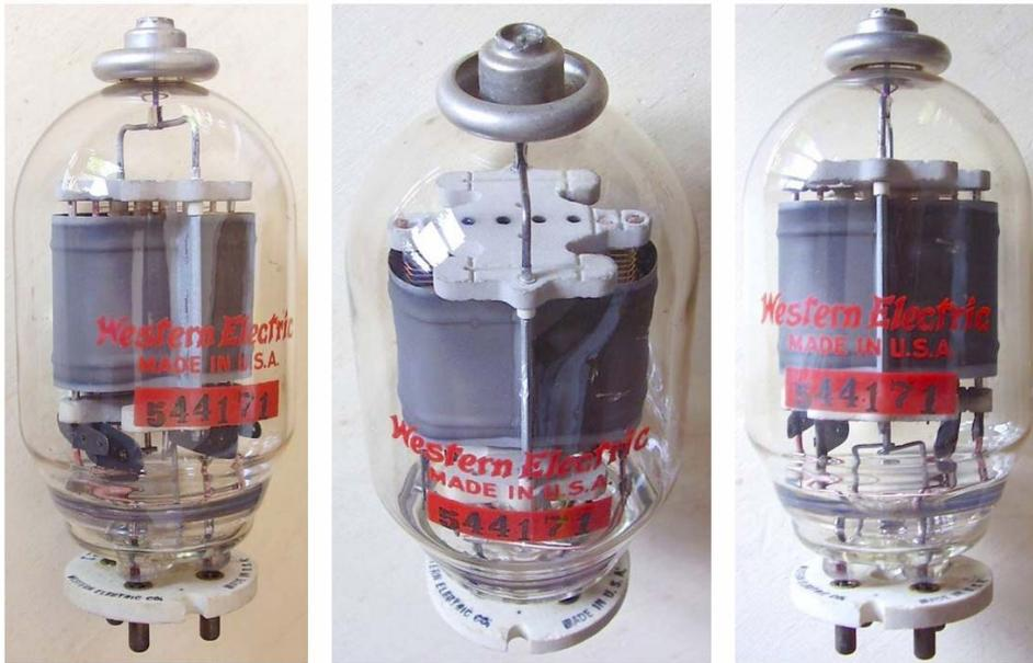
Pulse power tetrode intended for radar modulators. Up-rated 715B with corona guarding ring on plate cap and quad-in-line cathode structure. Grid cooling fins near the base connections.
