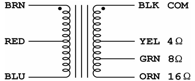
**NOTE:** ORIGINALLY DESIGNED FOR 3/7/15 OHM LOADS
