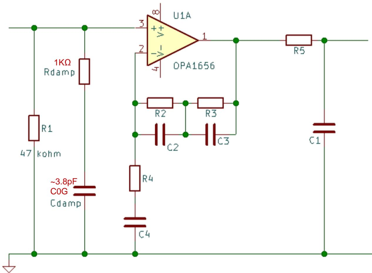
NOTE: Rdamp and Cdamp installed across RCA input connectors' signal and shield tabs.
