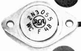
2N3055 115 watts @25°C TO-3 Package
