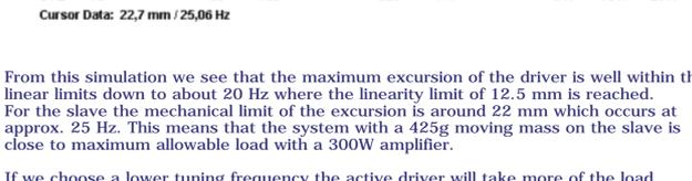
From this simulation we see that the maximum excursion of the driver is well within the linear limits down to about 20 Hz where the linearity limit of 22.5 mm is reached. For the slave the mechanical limit of the excursion is around 12.5 mm which occurs at approx. 25 Hz. This means that the system with a 425g moving mass on the slave is close to maximum allowable load with a 300W amplifier.
