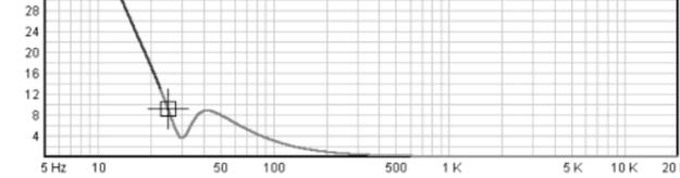
From the simulation it can be seen that the system response is up by about 3 dB at 25 Hz compared to the sealed box. We get about 104 dB with 300 W RMS at 25 Hz.
