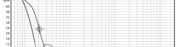
The cone displacement of both the passive and active driver is OK within the safe operating limits of the drivers. However it can be seen that the cone displacement rises steeply below 20Hz meaning that a high pass filter to protect against overload is highly recommended.
