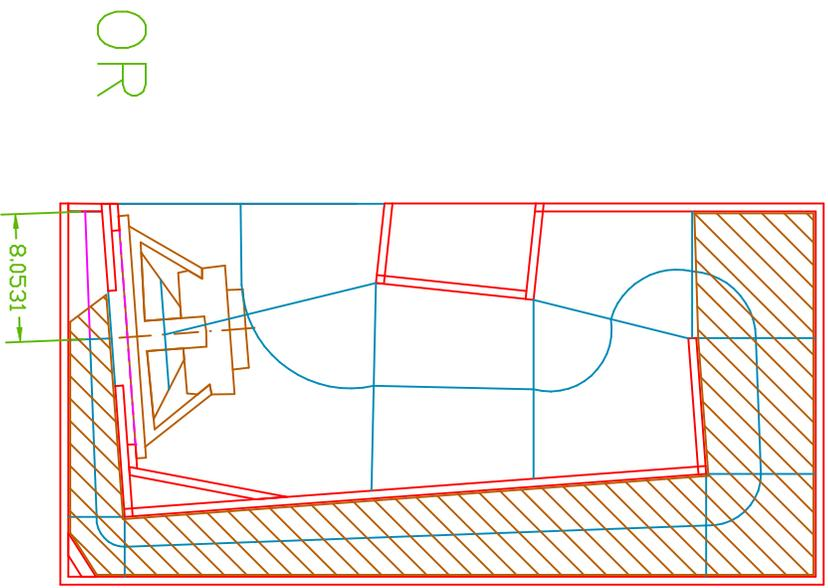
As drawn the speaker vents through a throat chamber into a 29" wide horn slot. Another possibility would be venting into a horn slot that widens from the speaker to meet the 29" width at the first right angle box corner from the throat. Obviously, it would be easiest to have the speaker coupled to the horn through a full size circular opening, e.g.: about 14" Dia. for the 401SLF.
