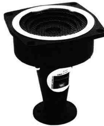
The JBL 2301 is a perforated plate acoustic lens for use above 1200 Hz. It is intended for use as the high frequency element in a two or three frequency band integrated system where the length of throw does not exceed 9 m (30ft). Above 1200 Hz, the pattern has a conical shape with an included angle of 90°. Sensitivity 109 dB. The 2301 will accept 25 mm (1 in) drivers only. Nominal Q=4 (2 kHz octave band).
