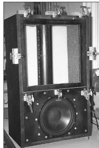
PHOTO 1: Test box showing the frame and toggle clamps for holding a test panel.
