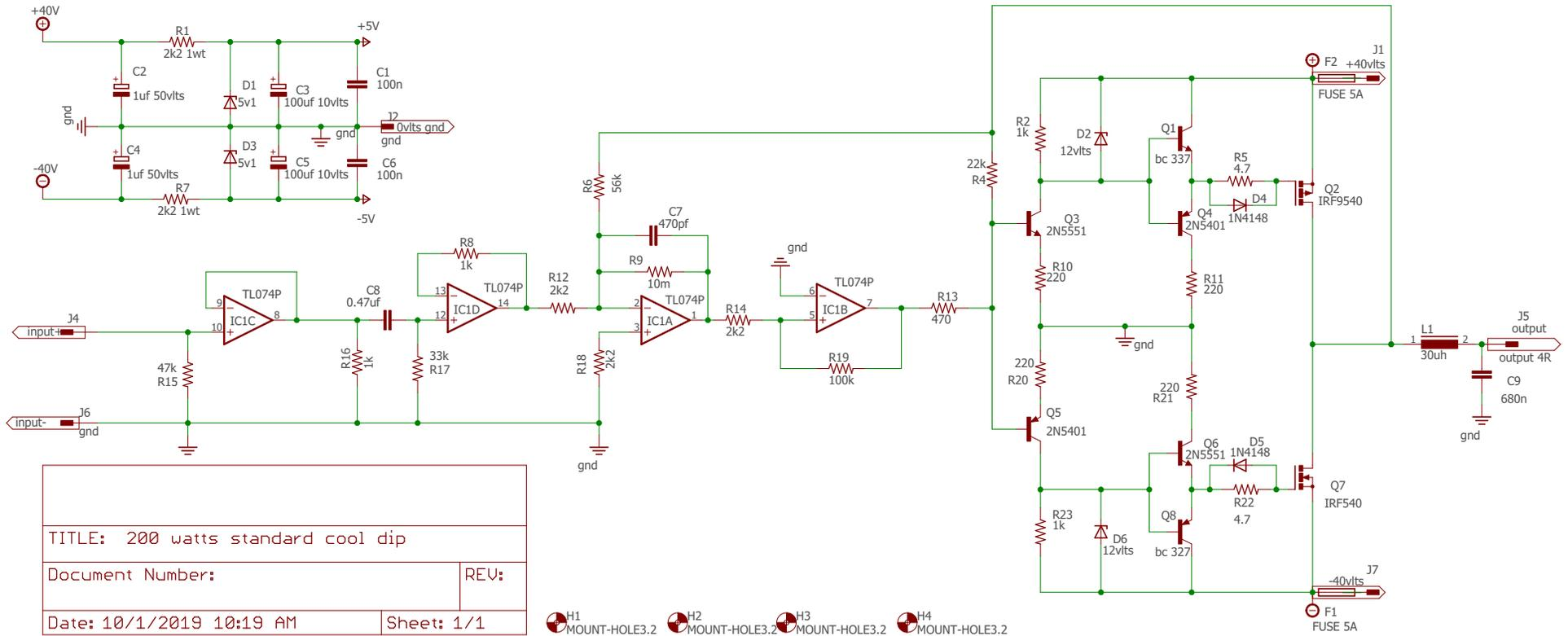
the configuration has been tested with 30uh output inductor (er 39 4mm gap with 22turns ) the load was 4 ohms played loud for some hours andworked well ,without a heastsink.
