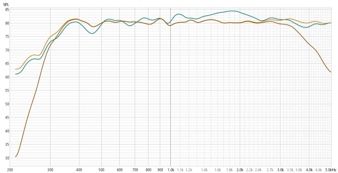
Mid 200-5,000Hz. Dark Green - Raw, Orange - Biquads applied, Brown - XO applied. XO LR 96 Hi Pass 290Hz, LR 48 Lo Pass 3800Hz
