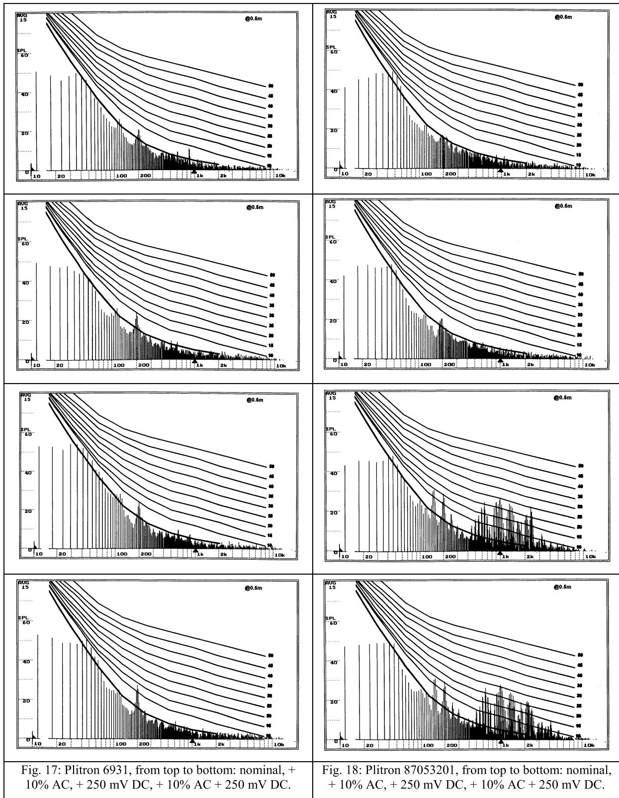
Fig. 17: Plitron 6931, from top to bottom: nominal, + 10% AC, + 250 mV DC, + 10% AC + 250 mV DC.
