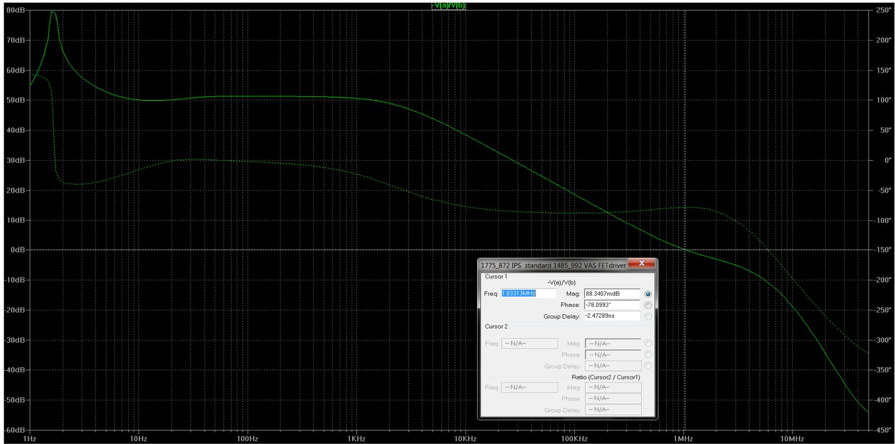
Open loop bandwidth with JUMPER closed
