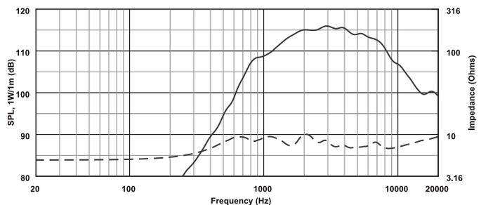
Note: Frequency response and impedance of the DH3/2010A driver attached to an HP64M Horn, measured on axis in the far field using one watt input (2.8 Vrms). SPL calculated to 1 meter equivalent by inverse square law.
