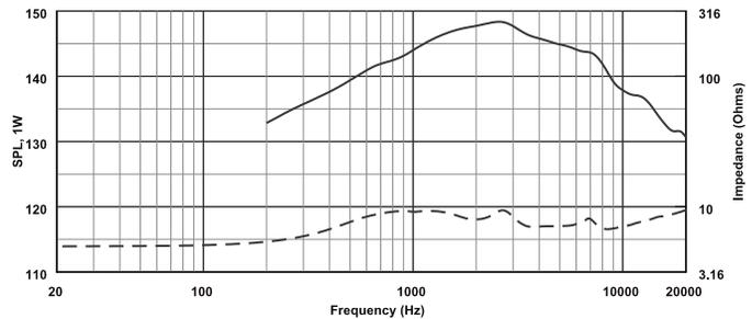
Note: Frequency response and impedance of the DH3/2010A driver attached to a 25mm (1.0") diameter plane wave tube, using one watt input (2.8 Vrms).
