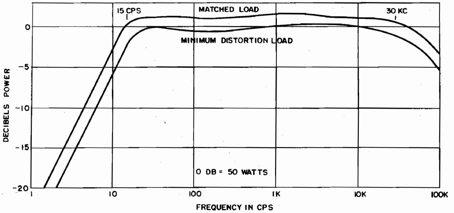
Figure 2. Maximum Undistorted Power Output vs. Frequency.
