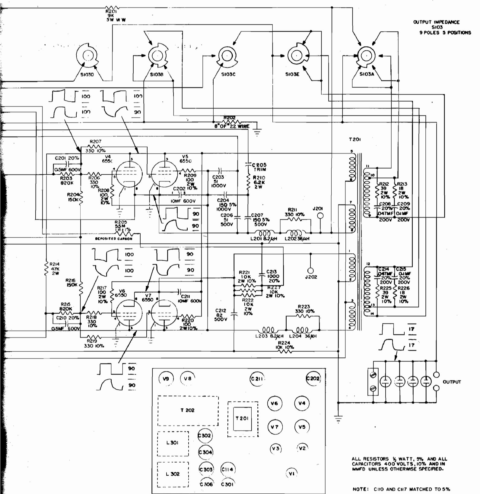
VOLTAGE MEASUREMENTS MADE BETWEEN PINS OF EACH SOCKET AND GROUND WITH V.T.V.M. ALL KNOBS IN MAXIMUM CLOCK WISE POSITION, LINE VOLTAGE SWITCH AT REAR OF CHASSIS IN HIGH POSITION WITH 119V. (LOW POSITION FOR 109V LINE). NO CONNECTIONS TO THE INPUT OR OUTPUT TERMINALS.
