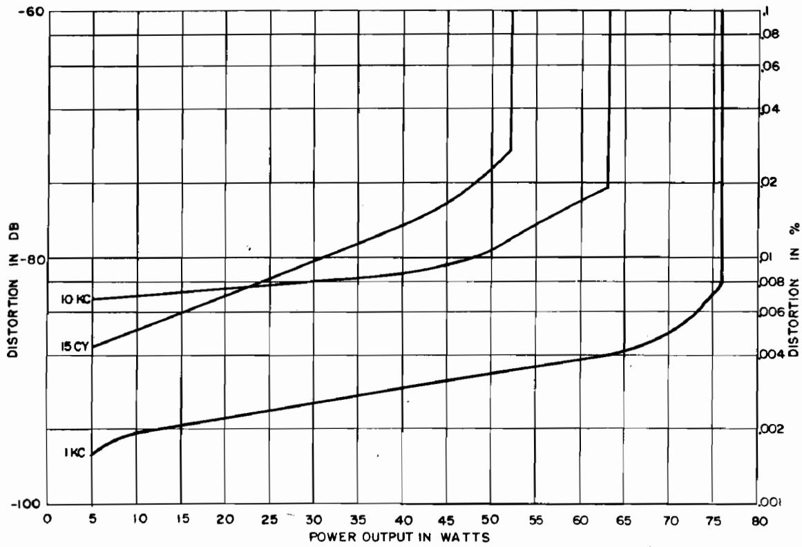
Figure 4. Distortion vs. Power with Matched Load.
