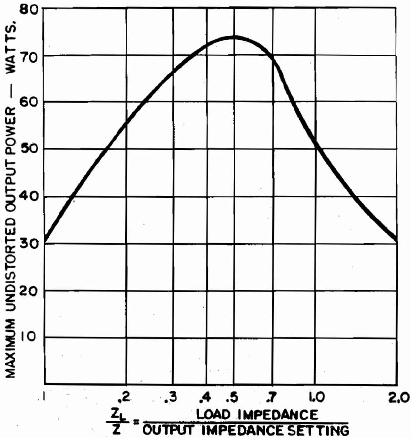
Figure 3. Maximum Undistorted Power Output vs. Load Impedance.
