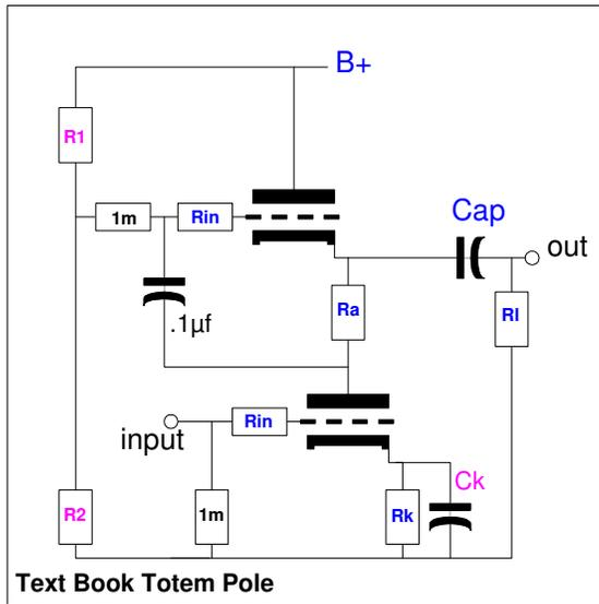
The textbook Totem Pole amplifier. Very popular. This circuit seems to promise it all. Low distortion, low  $Z_o$ , high gain. It works by using a top triode as a current source and a cathode follower at the same time. Resistors R1 and R2 set up the bias voltage for the top triode.
