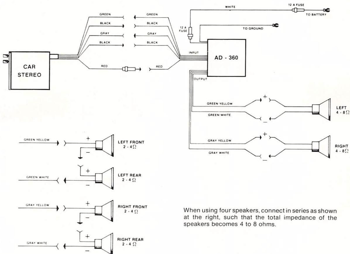
When using four speakers, connect in series as shown at the right, such that the total impedance of the speakers becomes 4 to 8 ohms.
