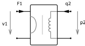
Figure 8 - Mechano-acoustical coupler
