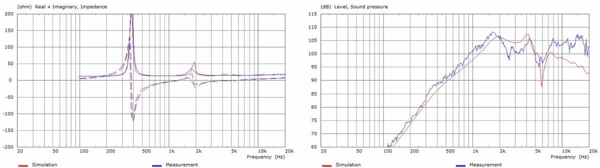
Figure 14 - Refined model: Electric driving point impedance and sound pressure level at 180 mm on-axis in front of aperture
