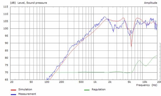
Figure 17 - Refine model. Weighted by normalized velocity distribution
