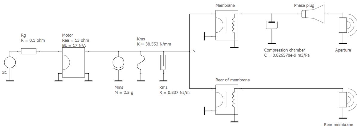
Figure 11 - Electro-mechano-acoustical network - simple modeling
