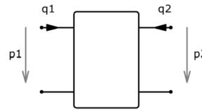
Figure 9 - Acoustic four-pole
