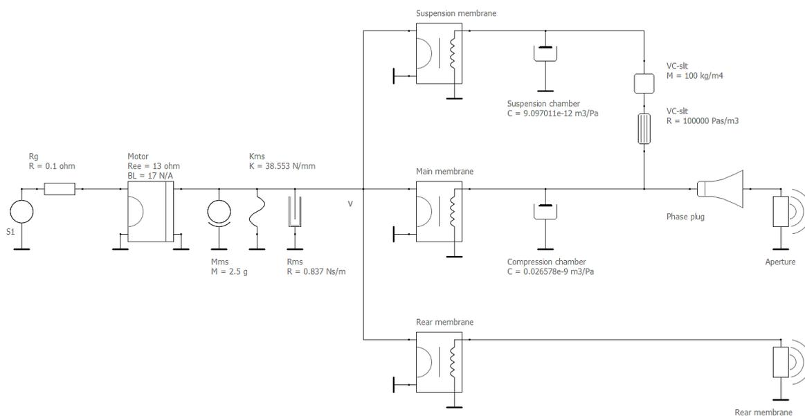
Figure 13 - Electro-mechano-acoustical network - refined model
