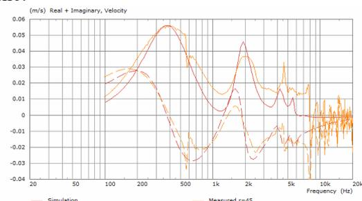
Figure 16 - Refined model: Mechanic velocity close to the voice-coil former
