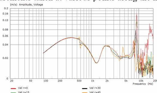
Figure 15 - Velocity distribution of main membrane Center at  $r = 0$ . Voice-coil-former at  $r = 45$  mm
