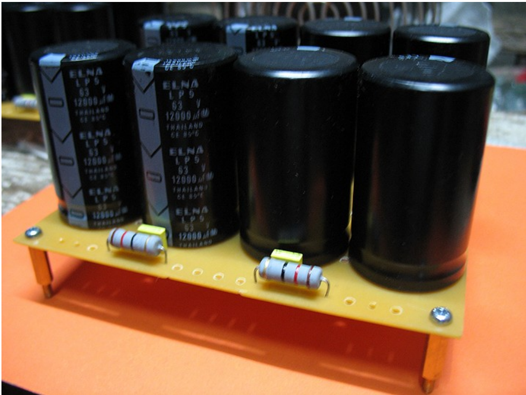
Wired and ready for testing. Notice I used two boards for a dual-mono approach in the PSU for the DA Honey Badger Power Amplifier prototype.
