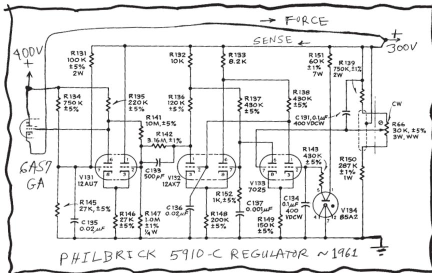
The 5910 dual regulator amplifier was built in a little boxy subassembly. The tubes stuck up above the box, with the passive components mounted on turret terminals along the insides of the box.
