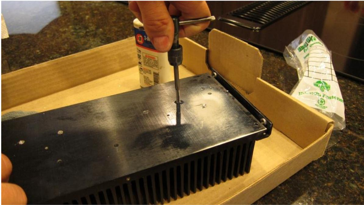
The photo, below, is of the drilled and tapped heat sink (again, the top three holes came in the sink and are not of use to us). I picked up some aluminum bar (1 inch X 1/4 inch) at the hardware store and cut a 10 inch piece, the same length as the board. The bar has been drilled to allow 10-32 screws to pass through it and into the threaded holes in the sink. Sorry for the lousy exposure.
