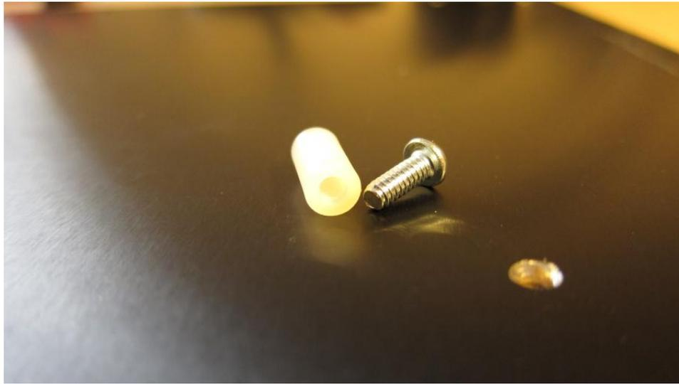
The photo, above, is a close-up of a 1/2 inch double-threaded nylon offset along with the 6-32 machine screw that were used to hold it to the bottom of the case. Another 6-32 screw went through the circuit board and into the top of the tap. Got these at ACE Hardware on a quick trip. We used them on the F5 and they were fine.
