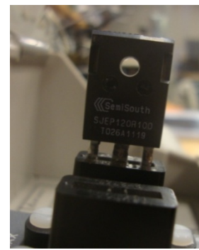
SJEP120R100. A JFET awaits trial by Curve Tracer. Is this really a good lie detector test?
