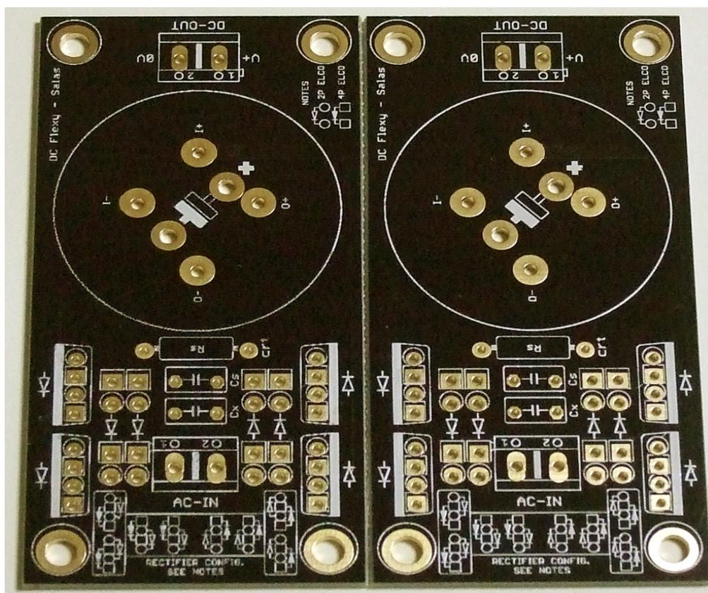
Accepts standard axial or TO-220 diodes. One or the other type may be used. Don't populate both together. Located at the board's sides the TO-220s can be bolted to chassis used as a sink if their temperature gets high. Their backs if conductive must be isolated with Silpads for allowing that.
