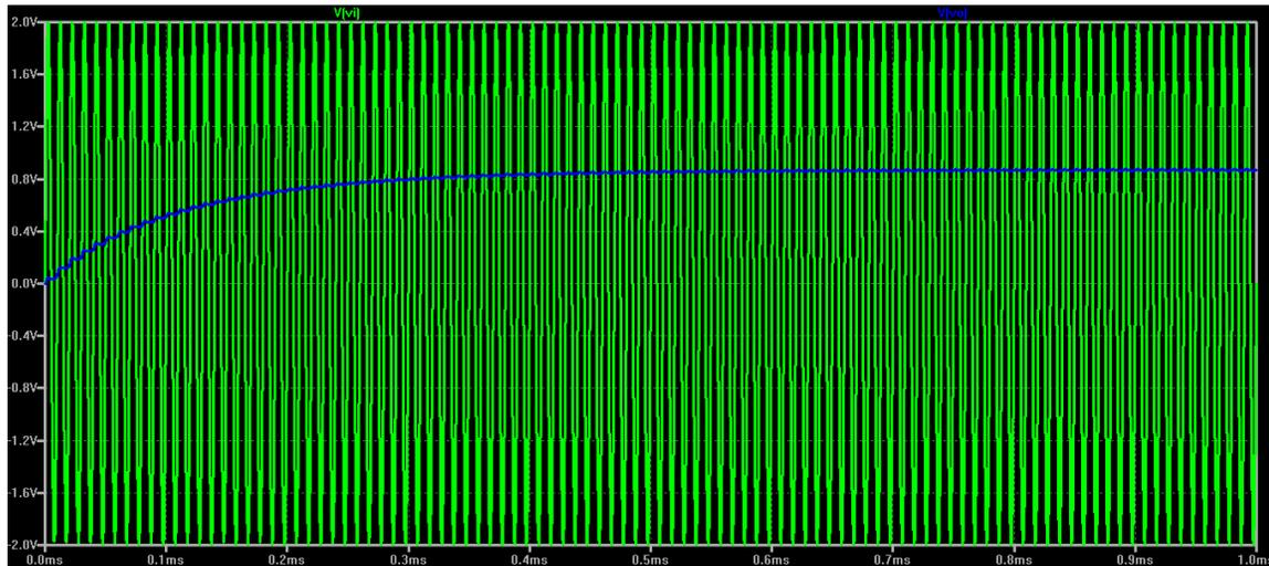
Figure 2 - Blue line is DC Output with 2V 100kHz Input Signal
