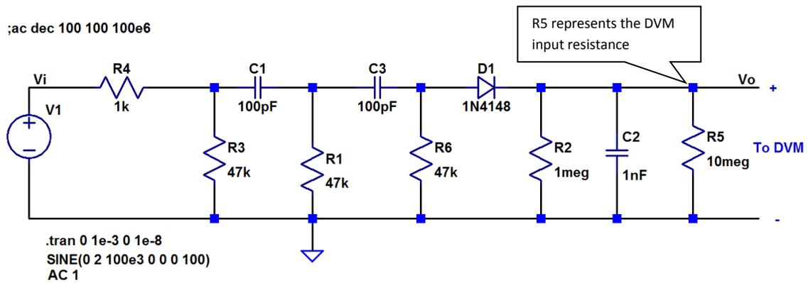
Figure 1 - Oscillation Sniffer Circuit
