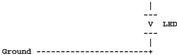
The idea of the circuit is that the digital data is fed through a series current limiting resistor to the LED (typically LEDs only require 5-30mA). A digital 0 is 0V and the LED is off. A digital 1 is +5V and the LED is on. That's it!
