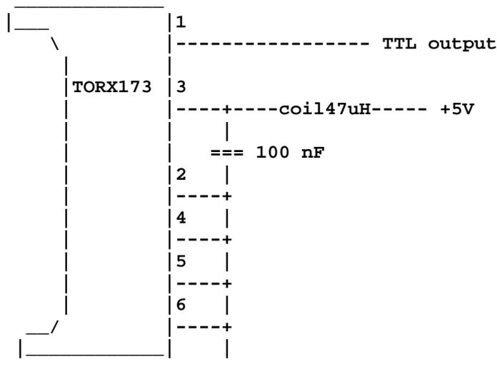
The 47 microhenry coil and 100 nF capacitor make a filter against digital noise in +5V power source. The Toslink receiving module used in this circuit is TORX173 from [Toshiba](#). This circuit is a part of circuit diagram from Elektor Electronics magazine issue 4/1997 page 66.
