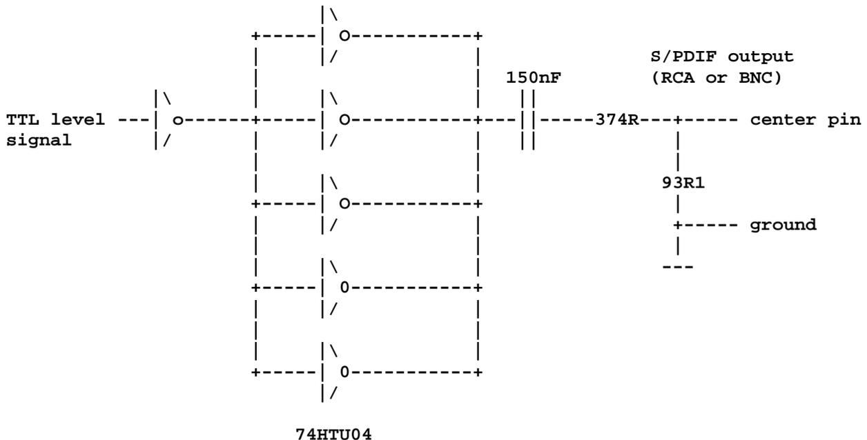
This circuit does not provide any isolation on the output. The TTL level signal from 74HCT04 buffer is attenuated to the levels specified in S/PDIF optical interface by using the voltage divider made of 374 ohm and 93.1 ohm resistors. This circuit is based on S/PDIF converter circuit diagram from Elektor Electronics magazine issue 4/1997 page 66.
