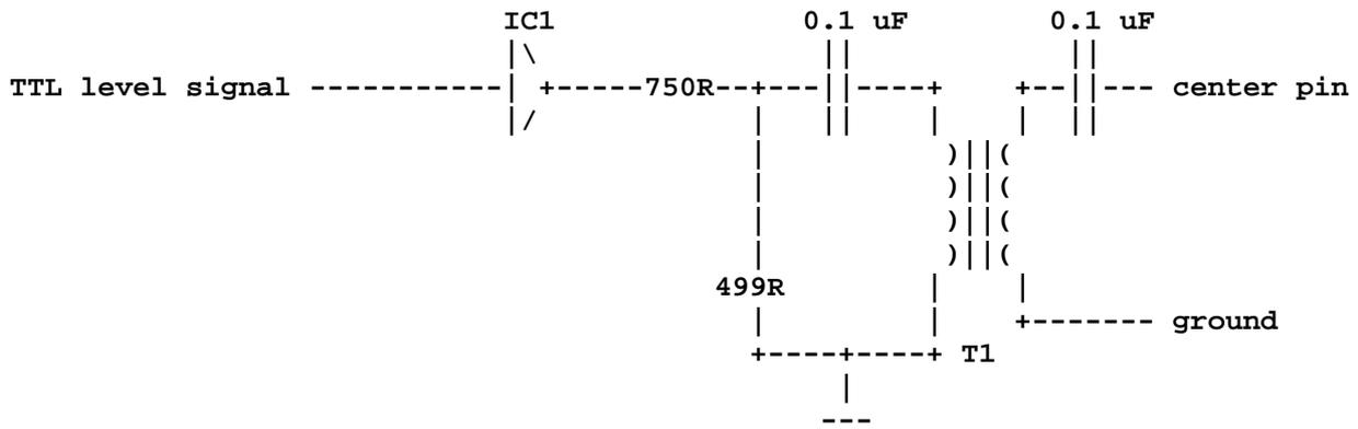
T1 is a HF-transformer which has 2:1 turns ratio. Transformer type used in example circuit is SC944-05. IC1 in this circuit consists of 8 parallel connected buffer ports from 74ACQ244 IC.
