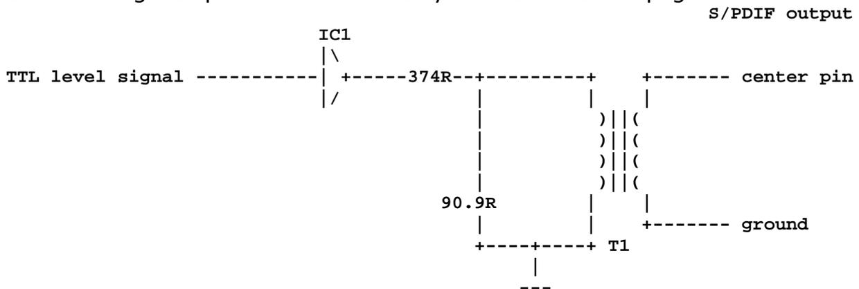
The transformer used in this circuit is 1:1 pulse transformer (the original application note suggested pulse transformer from Pulse Engineering or Schott Corporation). IC1 is a buffer IC which must be capable to supply enough current to drive the 75 ohm S/PDIF interface to full voltage swing specified (capable of loading 415 ohm load or capable of supplying 12 mA current).
