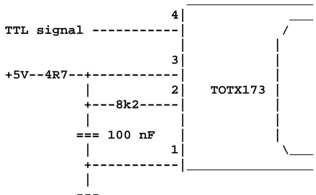
The 4.7 ohm resistor and 100 nF capacitor make a filter against digital noise in +5V power source. The Toslink transmitting module used in this circuit is [TOTX173](#) from [Toshiba](#). This circuit is a part of circuit diagram from Elektor Electronics magazine issue 4/1997 page 65.
