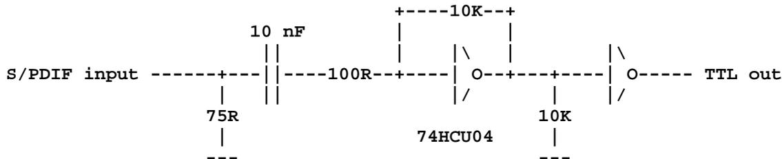
This circuit is part of circuit "Splitter for S/PDIF coax/optical output" by T. Giesberts from Elektor Electronics magazine July/August 1995 pages 78-79. The chip 74HCU04 is manufactured by [Philips](#)
