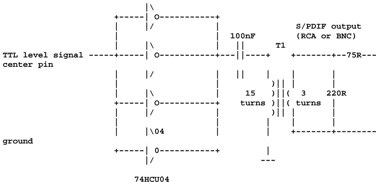
This circuit is part of circuit "Splitter for S/PDIF coax/optical output" by T. Giesberts from Elektor Electronics magazine July/August 1995 pages 78-79. The transformer T1 is made to G2.3-FT12 ferrite ring core. Primary coil is 15 turns of 0.5 mm diameter enamelled copper wire and secondary is 3 turns of 0.5 mm diameter enamelled copper wire. The chip 74HCU04 is manufactured by [Philips](#)
