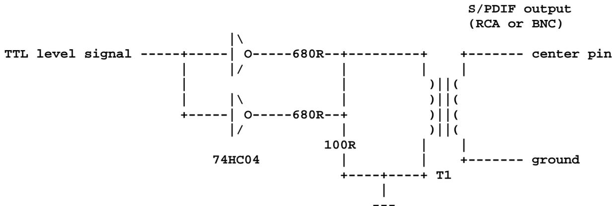
Idea for this circuit is taken from "A digital Output for the CD720" web page (was at <http://www.spiceisle.com/homepages/brian/audioidy/mods/digi-out.htm>). The transformer T1 is high quality 1:1 pulse transformer (can be salvaged from old broken network interface card or similar source).
