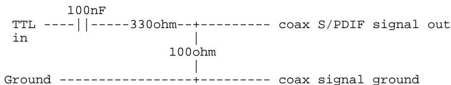
This circuit interfaces directly to the TTL level output provided by some sound equipment (CD-ROM or soundcard). This circuit works if the equipment which gives out TTL level has powerful enough TTL output to run this circuit (enough current output capability). If this simple circuit does not work reliably, then you need to build a circuit which includes the buffering electronics.
