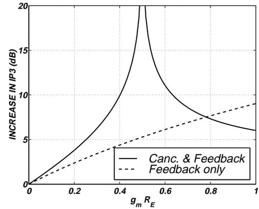
Figure 4: Increase in output-referred IP3 in common-emitter amplifier.
