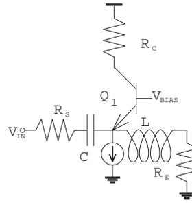
Figure 3: Simplified common-base amplifier.
