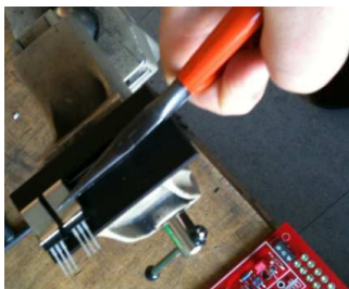
Mounting the power transistors
