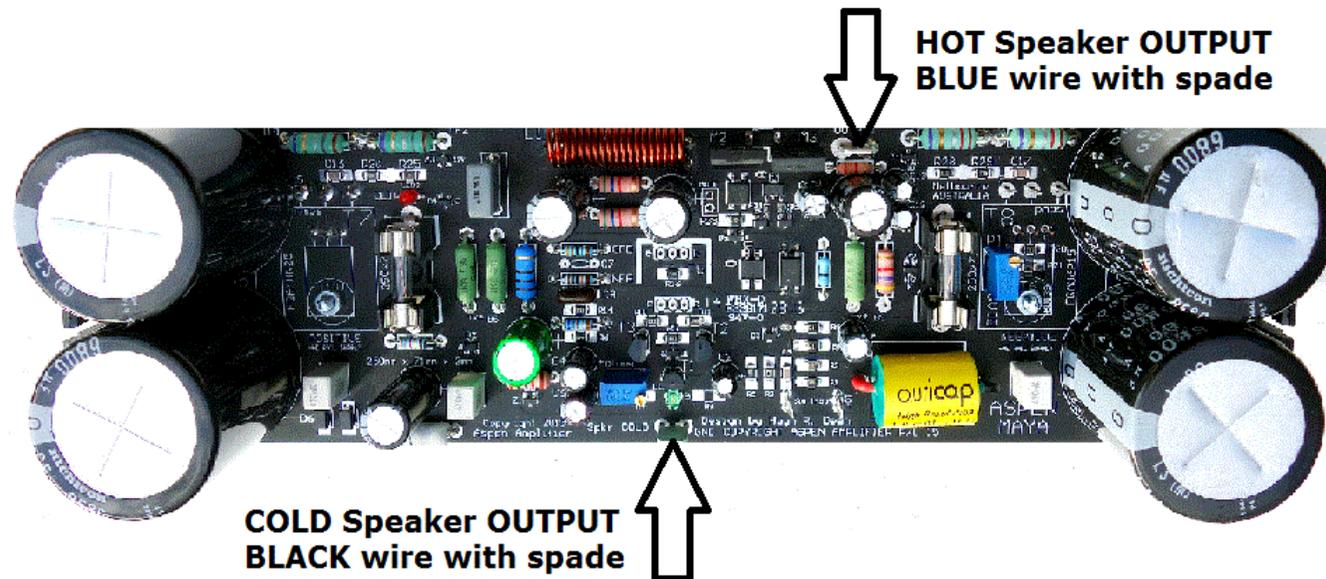
The Maya 200 is not fitted with short circuit protection but it is fitted with mains and rail fuses (all 15A) and speaker DC protection using ultra-fast solid state relays. If the amplifier output is accidentally shorted to ground, then one of the fuses will swiftly fuse, and the protection circuit will immediately disconnect the speaker to prevent damage. Nevertheless, speaker leads should NEVER be shorted at any time, so when connecting speaker the amplifier MUST be turned OFF.
