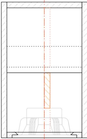
Install the brace second. Check for fit around the driver.
