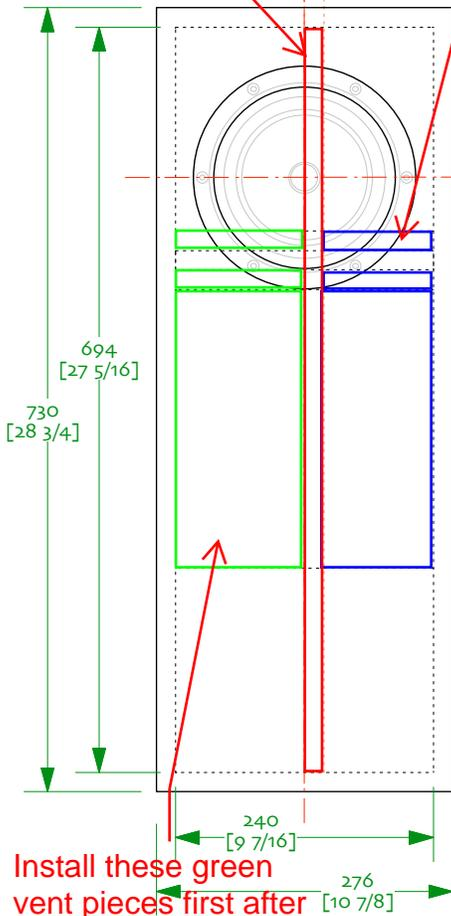
Install these green vent pieces first after the front, back, top, bottom have been attached to one of the sides.
