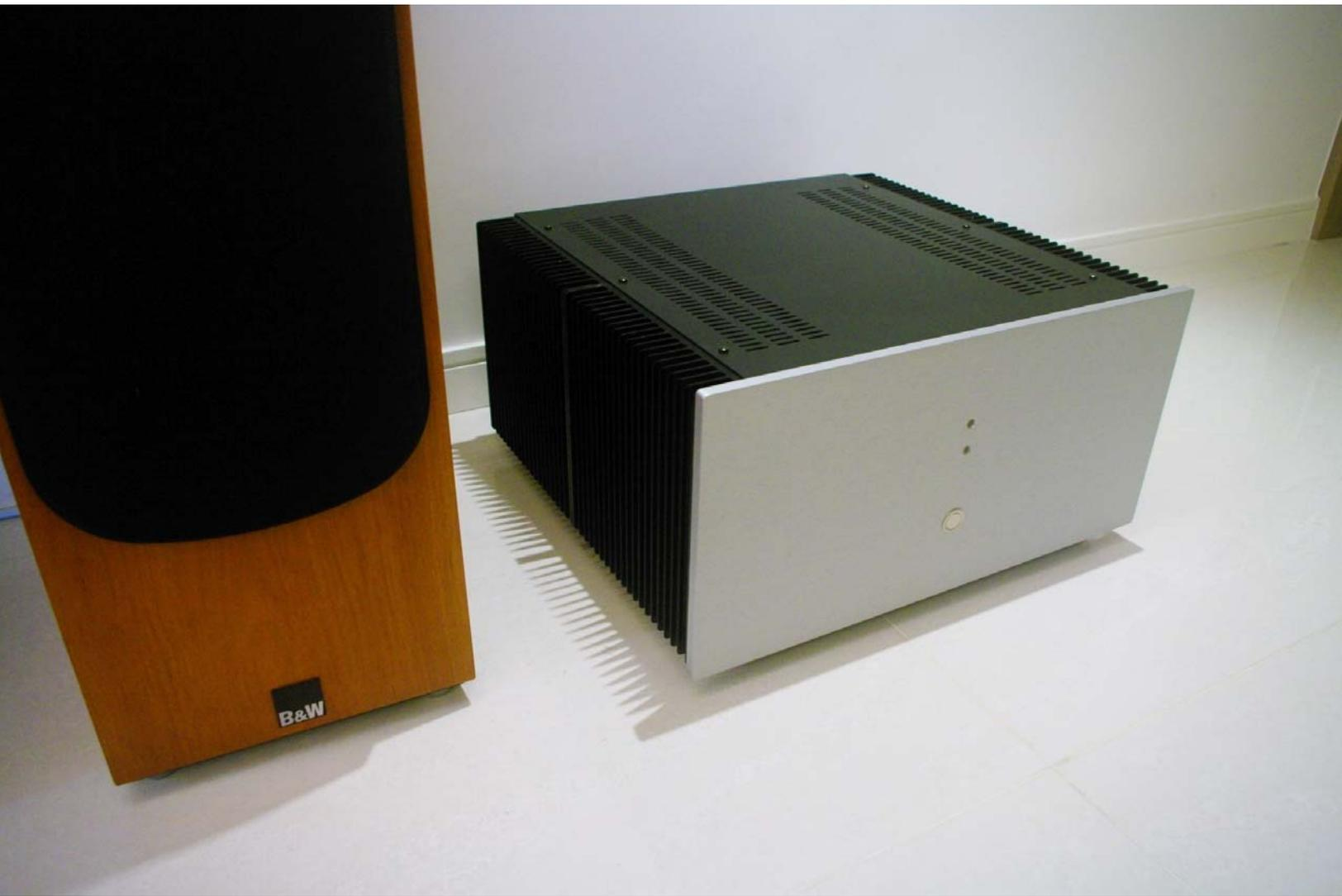
180 W RMS per channel [‘e-Amplifier’](#) featuring VFA topology, 10ppm 20 kHz distortion and peak output currents of  $\sim 40A$ , 3 Hz to 200 kHz bandwidth, and better than -100dB noise and hum ref 2.8V peak output into 8 Ohms that uses the wiring techniques described in this document.
