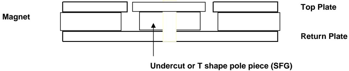
Suppose Top Plate thickness is 9 mm & the voice coil length is 20 mm
