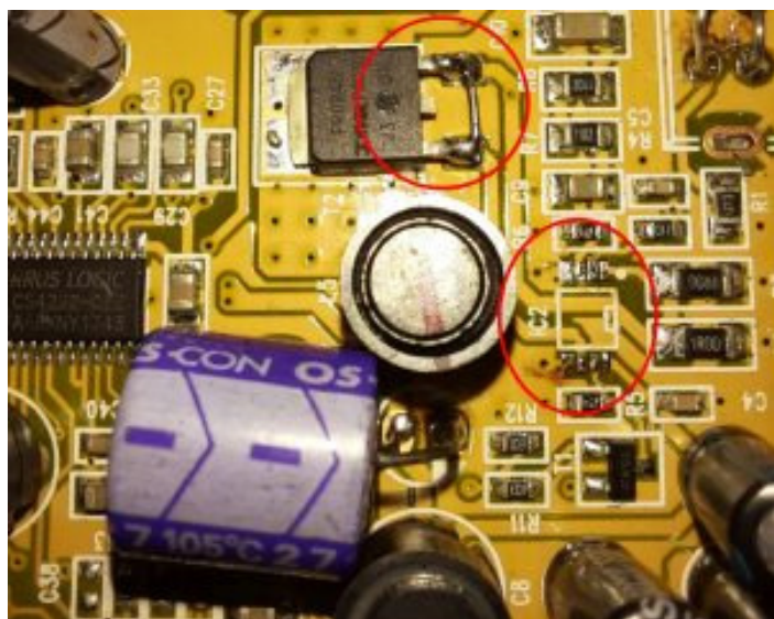
Disabling the 48V phantom power supply: removal of IC2 and Gate and Source of T2.
