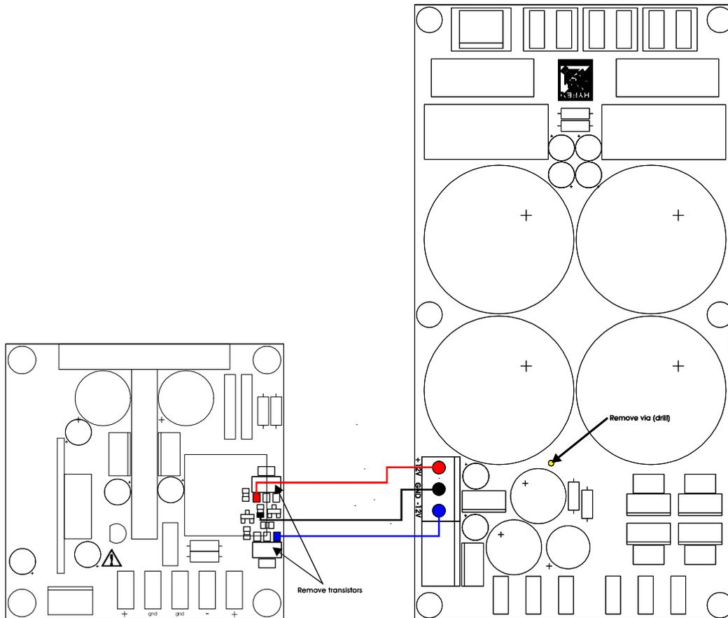
Connection diagram auxiliary supply/UcD180. **TOP VIEW.**
