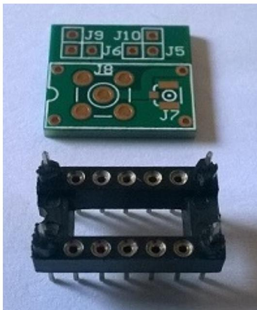
PCB ready to solder with the pin headers.
