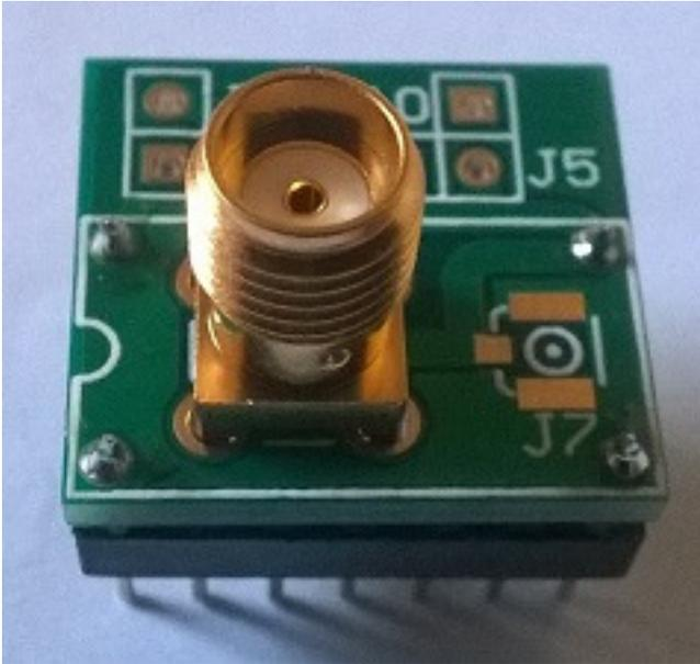
Finished board using pin strip header for direct soldering.
