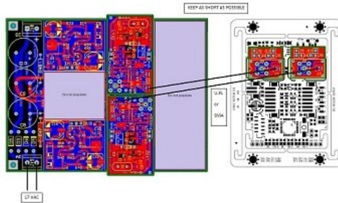
Option 2: fit 2 TWTMC-C XO directly on the TWTMC-DIL adapter board, then connect the power supply of the XOs to the TWTMC-D&D daughter board regulators. Keep power supply cables as short as possible. **Pay attention to the polarity of the power supply of each board.** You don't need to populate the switching logic and the dividers/delay of the daughter board.
