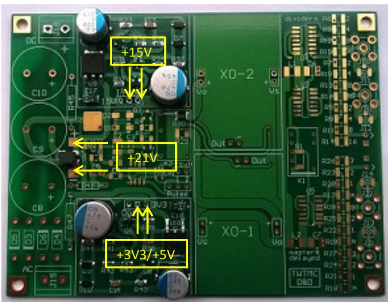
If you own a lab power supply, you can test the output voltage of the regulators with a DMM.
