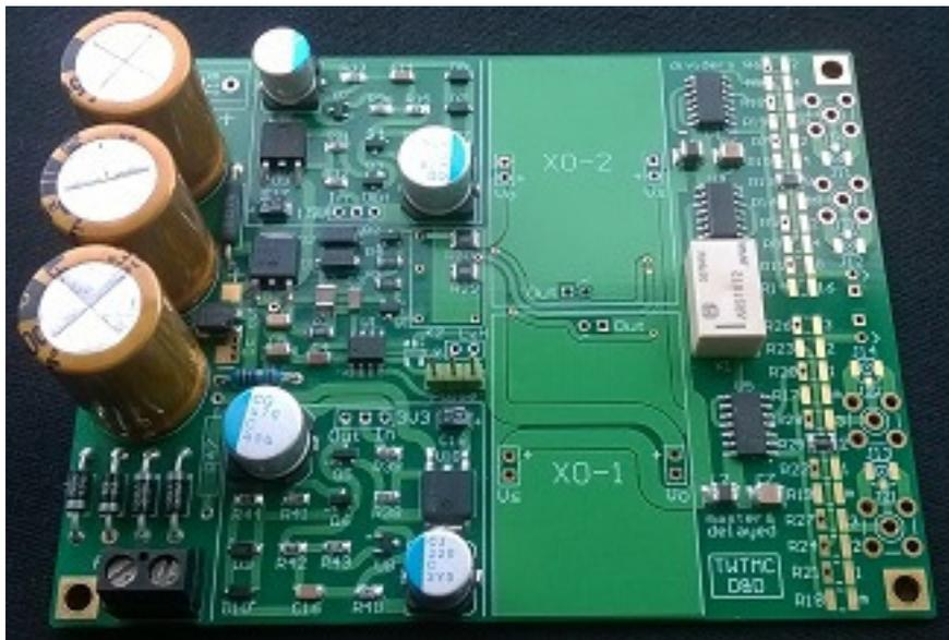
Dual XO switching, power supply, dividers and delayed clock
