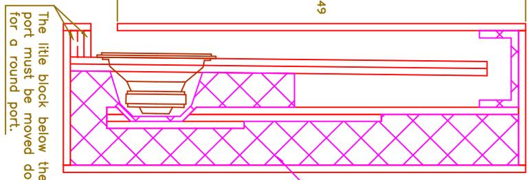
Derived from T-TQWT by bjorno for permco:
