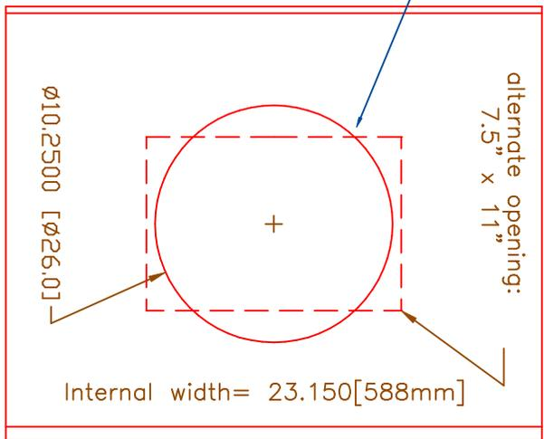
driver mounting baffle w/ S2 sized opening
