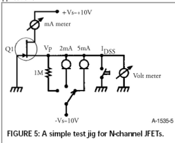
FIGURE 5: A simple test jig for N-channel JFETs.
