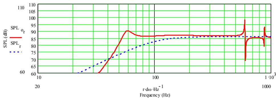
This one will require less stuffing to dampen the peaks in the treble, but there is also a peak at 60 Hz to take care of.
