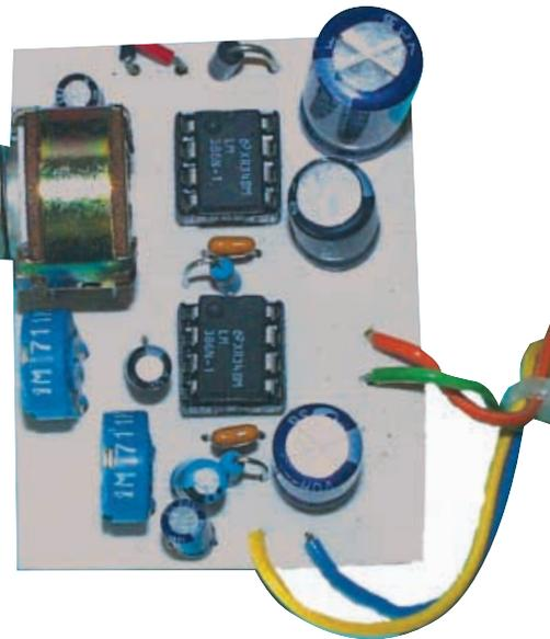
Fig.4. Interwiring for the "stand-alone" version of the Headphone Monitor. The sleeve connections for the jack socket and phono sockets must make a good "earth" (0V) with the metal case
