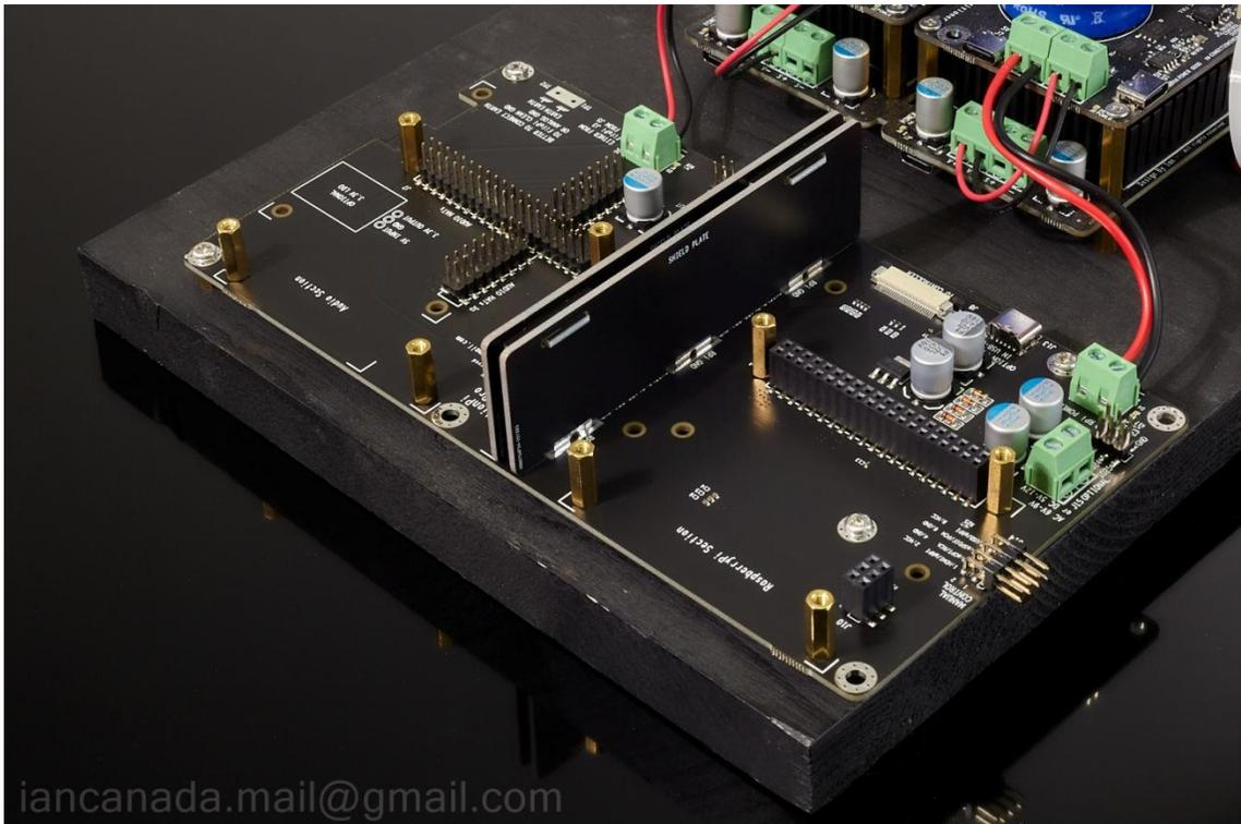
4. Assemble 4 of the **11mm** M2.5 standoffs to the daughter board and then install the daughter board the J1 of the StationPi PCB. Install a FifoPi or other audio HAT to J7 or J2 according to the orientation requirement of the project. Don't forget the connecting a 3.3V power supply for the FifoPi clean side or the other audio HAT.
