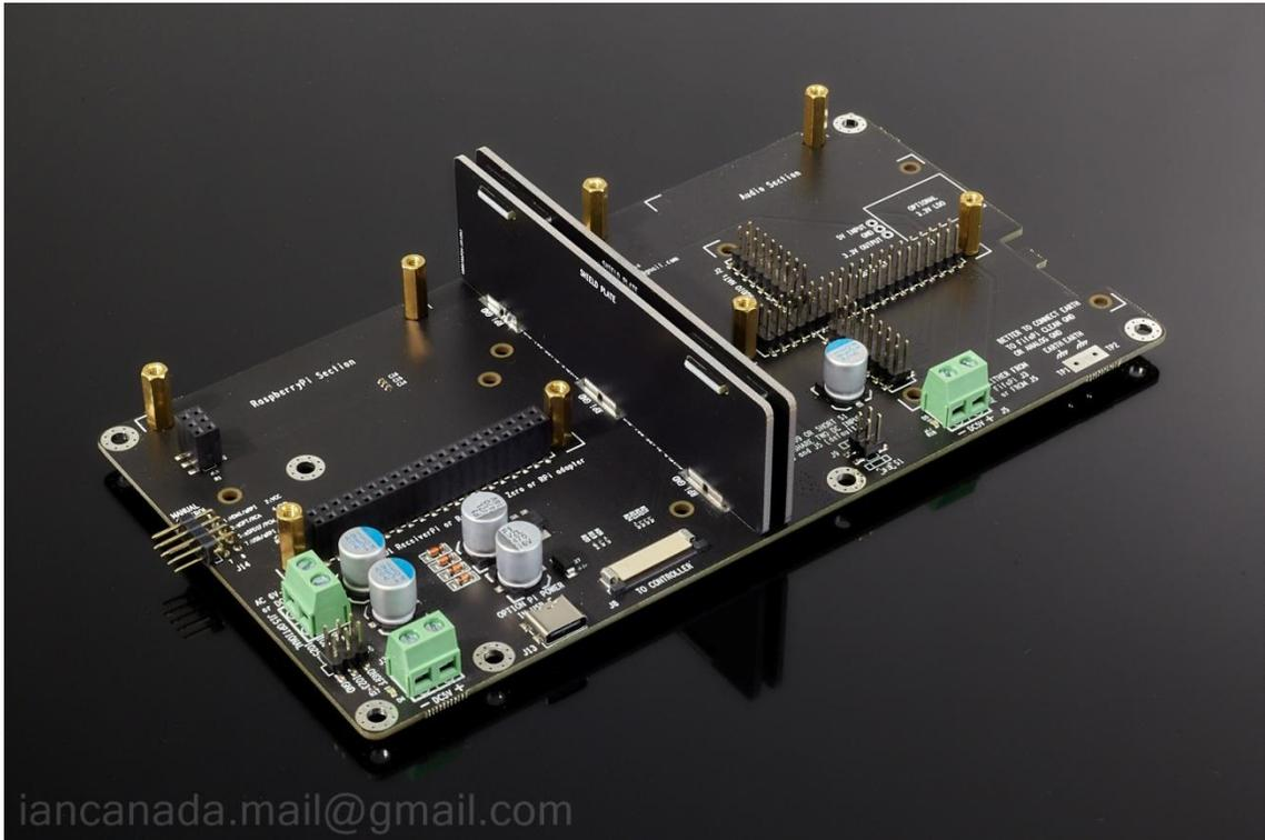
3. Mount the StationPi Pro PCB to the case/base using 4 or 6 M3 standoffs and screws. Connect a 5V RPi power supply to J3 or J13 (in USB-C). And connect a 5V audio power supply to J5. (Please see the application notes if you want to share one 5V power supply for both)
