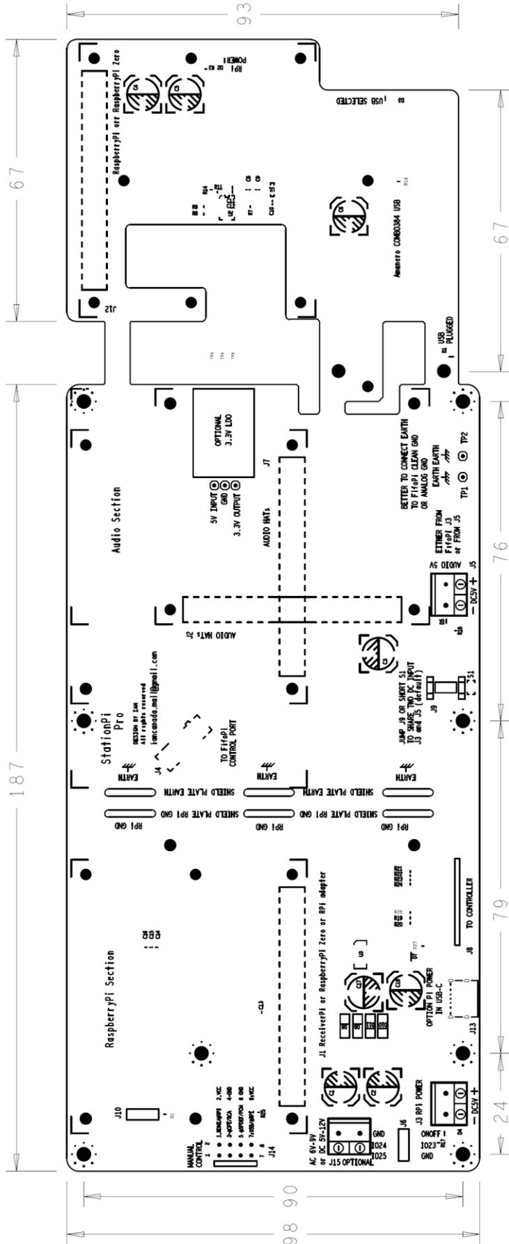
2. Install 8 13mm M2.5 standoffs to the StationPi PCB. If it is required, you can solder the two shield plates to the StationPi Pro PCB (just optional). Please use the spacer bits to separate the two plates well.
