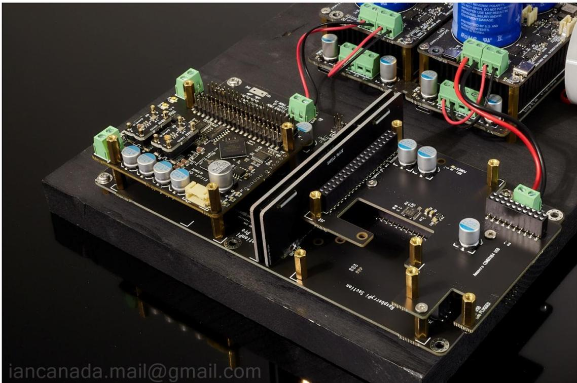
5. Install a RPi 4 /RPi 3 /RPi Zero 2 to the J12 on the daughter board. Install a TransportPi or a HDMIpi or other DAC HAT on top of the FifoPi. If it is required, install a Amanero size USB streamer directly to the daughter board (optional). Please see application note for how to select between RPi and USB as audio sources.
