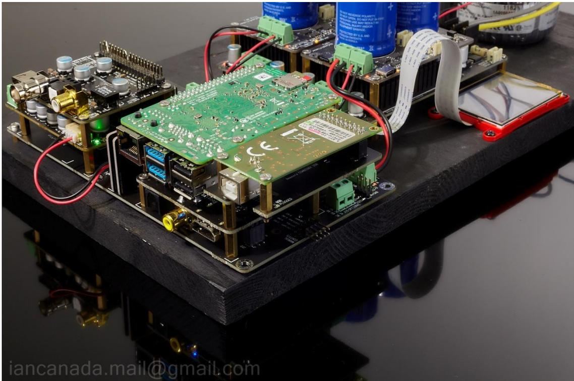
7. The StationPi Pro controller will be an independent open source project. It makes use of a 4D System GEN4-ULCD-24PT or GEN4-ULCD-24PT as the touch screen display. The StationPi Pro controller can also work as a FifoPi controller when an additional control cable is connected between FifoPi and the StationPi
