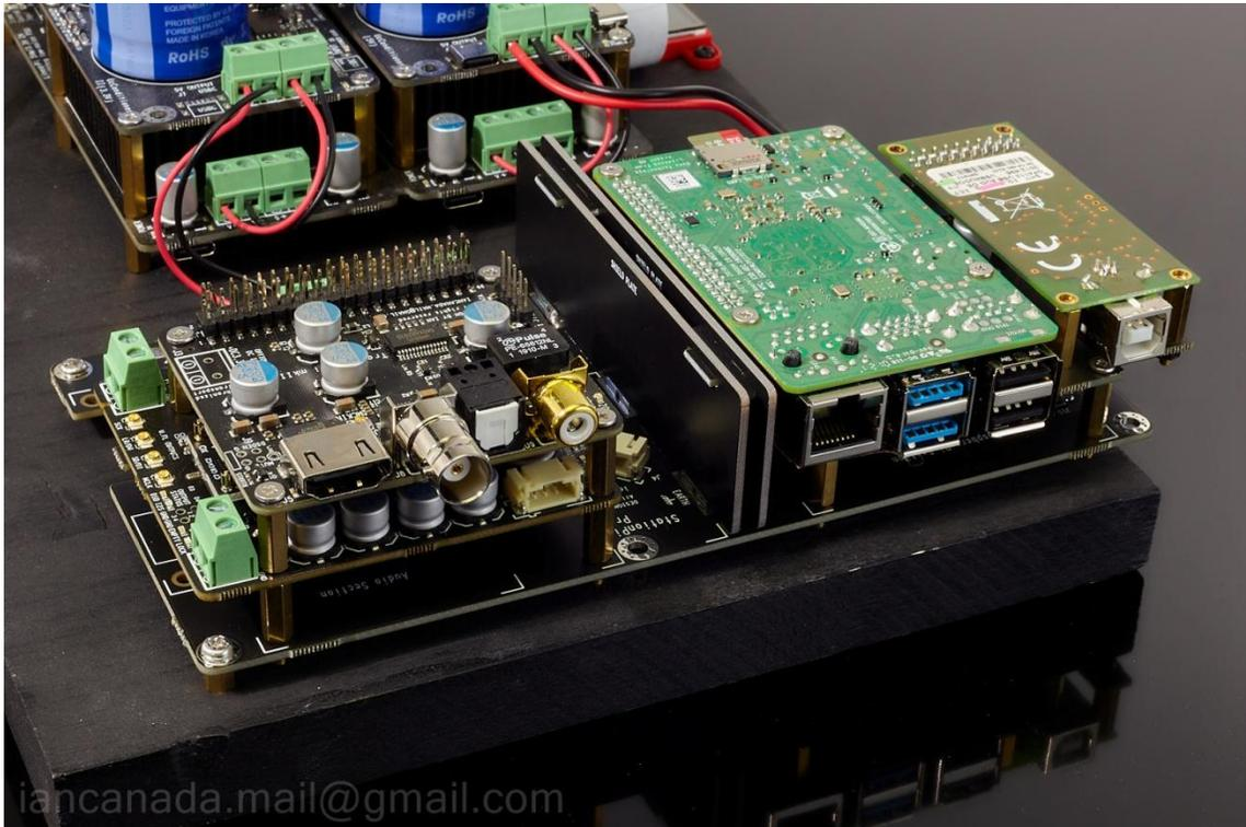
6. For a more advanced configuration, you can also install a ReceiverPi Pro underneath the daughter board. In this case, we will have five digital audio sources: RaspberryPi, RCA, optical, HDMI and USB. You can manually switch between them by J14 jumper settings or automatically by a touch screen StationPi Pro controller which can be connected to J8
