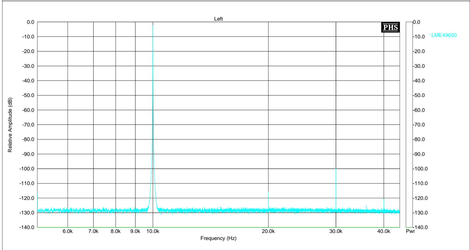
DAC output connected to buffer input. Buffer output connected to ADC input. BW pin connected to -V.
