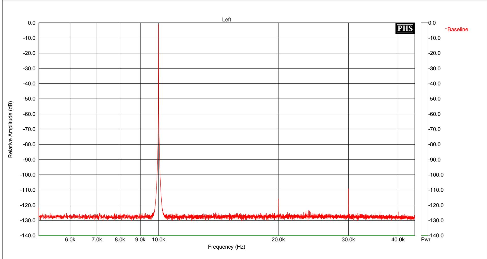
DAC output connected directly to ADC input.
