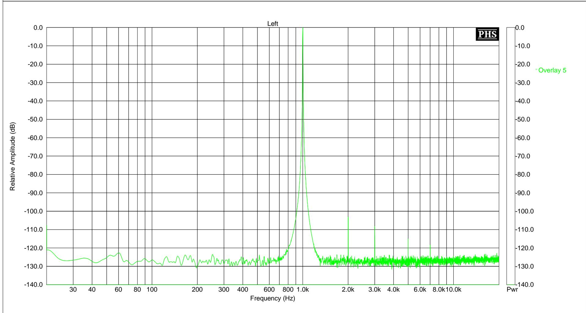
DAC output connected to buffer IC input and buffer IC output connected to ADC input. BW pin connected to -V through 220 ohm resistor.
