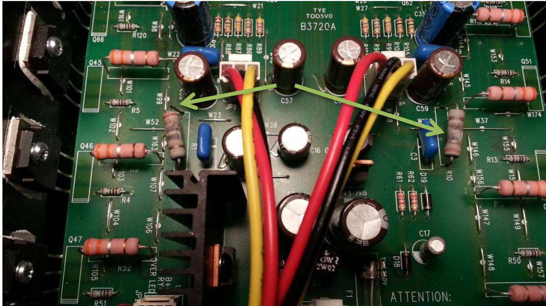
Damaged resistors at speaker output
