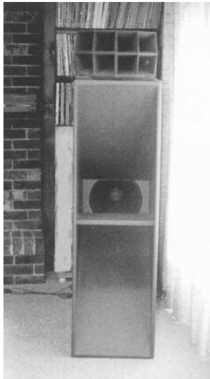
Right—Single 15" modified 210 with early wood 808 horn/802 driver
