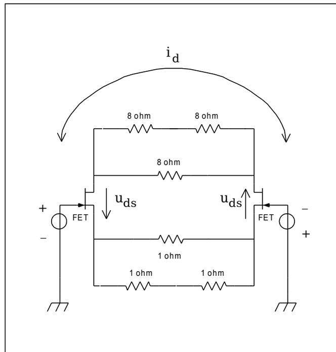
Replacement of the 8 ohm resistors:
